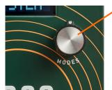
Press and hold the MODES button while powering up the pedal.
