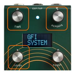
Push the knob's button to toggle the parameter mapping.
