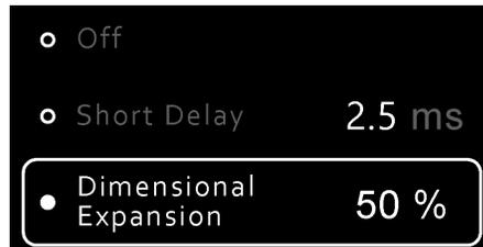
The stereo expander is useful only with **Mono-In/Stereo-Out** or **Dual-Mono (Stereo-In/Stereo-Out)** routing configuration. It should not be used when **Stereo-In/Mono-Out** routing mode is used.
