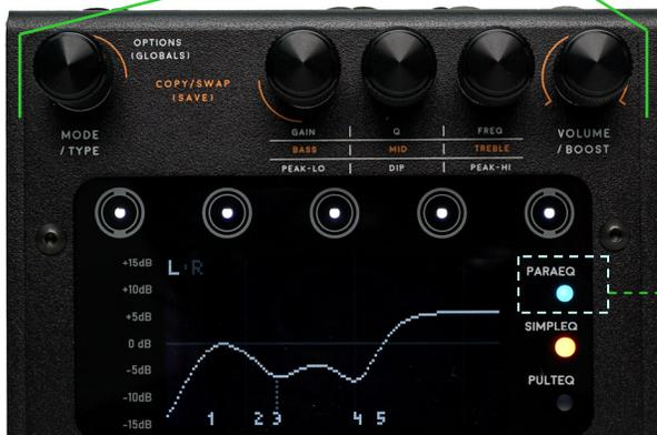
Parametric EQ now has control over the parameter knobs.
