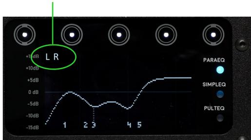
'L is highlighted, and R is dimmed' indicates that the two EQ channels are independent, and channel-L currently owns the *channel focus*.
