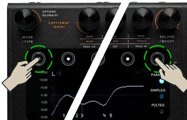
Hold for about 2 seconds to switch channel focus to the Right channel.
