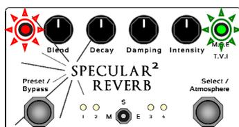
As long as you hold the footswitch down, the intensity parameter stays at its maximum value and both LEDs keep on flashing.
